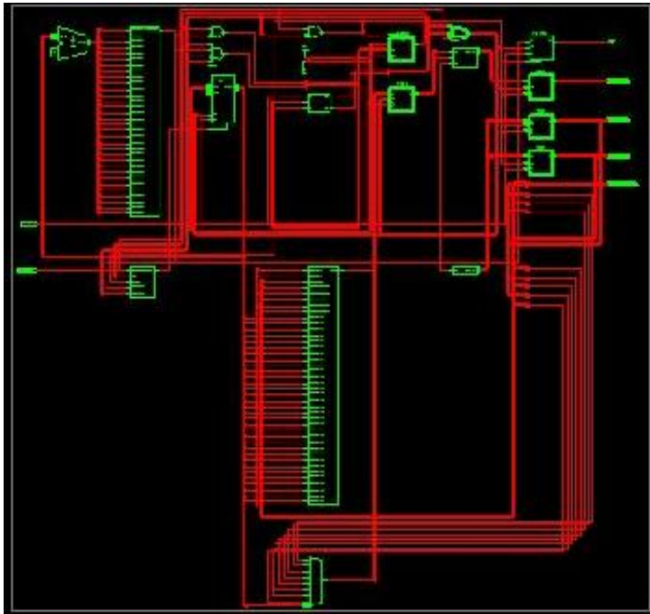
Fig. 5 RTL schematic view of \pi/4 QPSK Modulator
