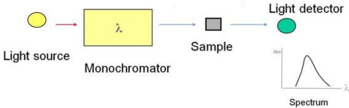
Fig.1. Block diagram of spectrum generation
