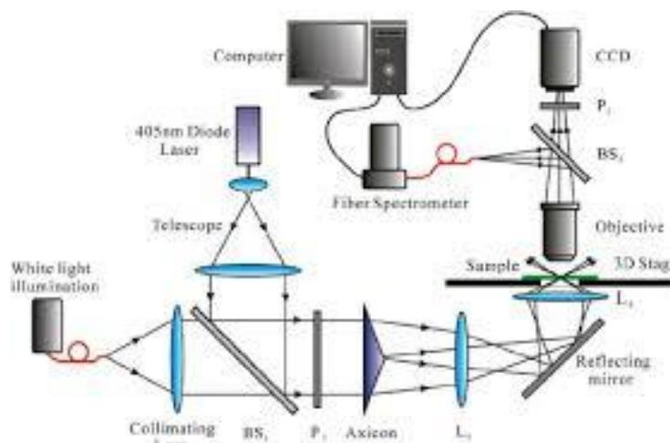
Fig. 4. Geometrical arrangement of optics
