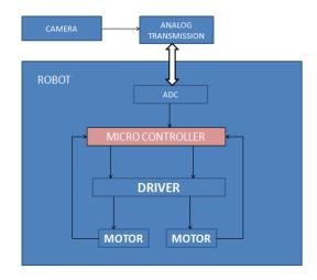
The above diagram shows the overall view of the color tracking system. It uses a camera, basically an android phone camera to capture the image. An object color is identified by the android application and a corresponding analog signal is generated. This analog signal is fed to the ADC and a digital signal is obtained as output at the micro controller. The micro controller facilitates the control of the two motors using a driver circuit and helps in the navigation of the robot to the target.
