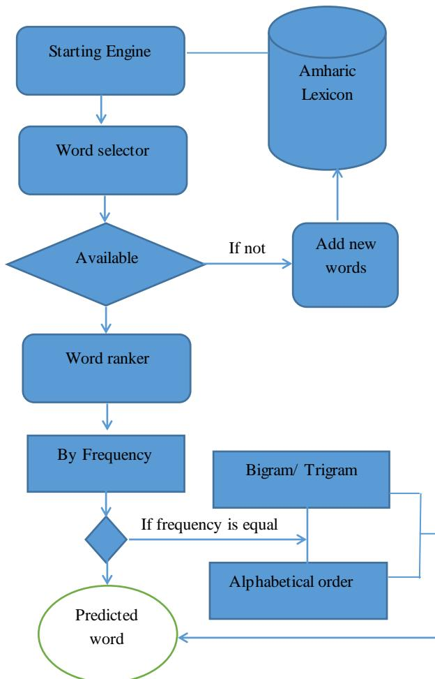
Figure 3.1 Architecture of the system
