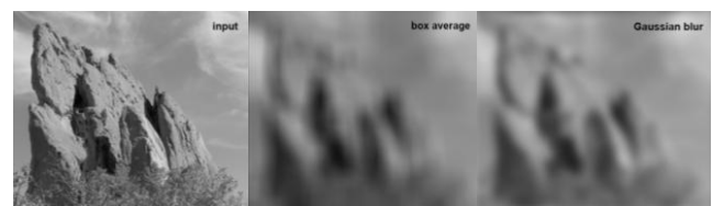
Fig. 6 Example of Gaussian Filter
