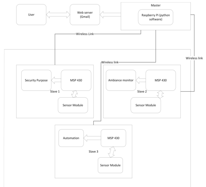
Fig. 1 Block Diagram of the proposed system for security purpose and to control the flow of water.
