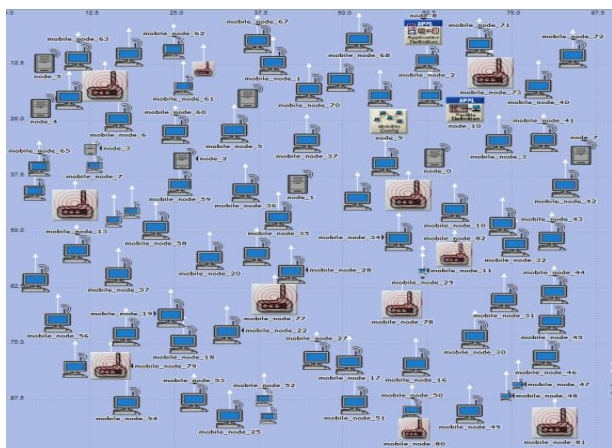
Figure 3: Jamming attacks scenario in MANET
