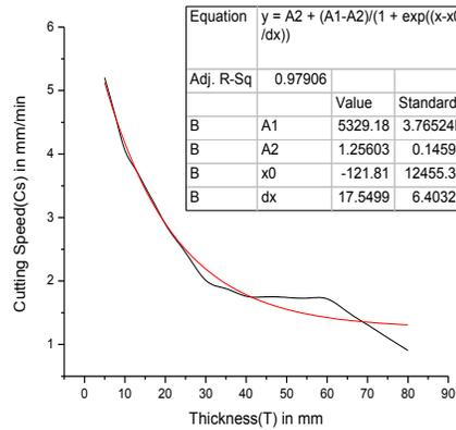
Fig.4 Effect of thickness on cutting speed
