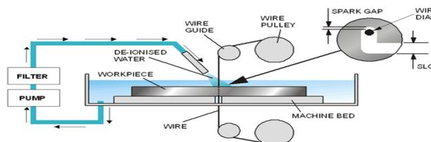
Fig.1 Machining in Wire EDM
