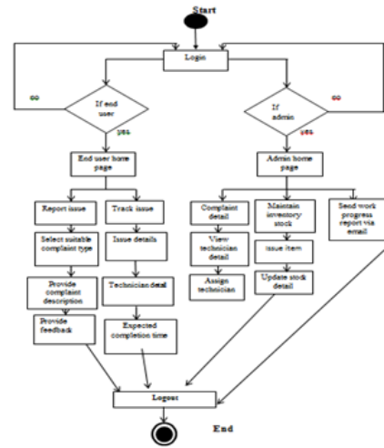
Figure3: Control flow diagram of web applications
