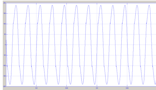
Fig.16 Source current after installation of shunt active filter system
