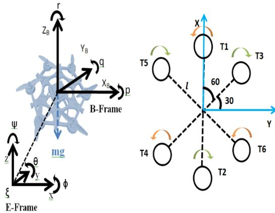
Fig 1. UAV Hexacopter structure and Frames.
