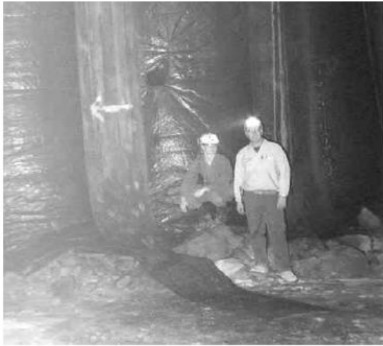
Figure 5. Used mine conveyor belt supplementing conventional mine brattice in a stopping.
