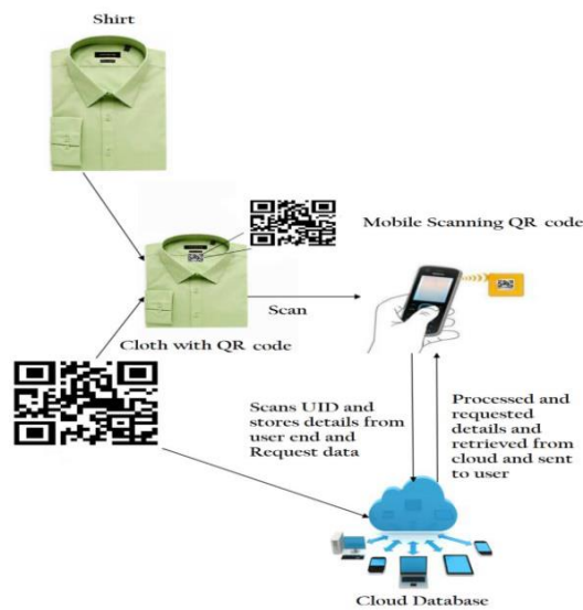
Fig.2 Basic Working of the System
