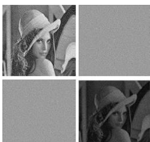
Fig. 1 Examples of visual cryptography (a) Original image, (b) and (c) over layered encrypted, (d) the superposed (b) and (c) giving the result.
