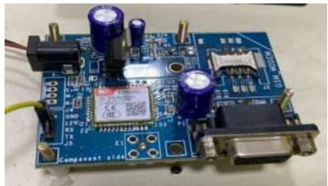
Figure 3.1.4: GSM Modem
