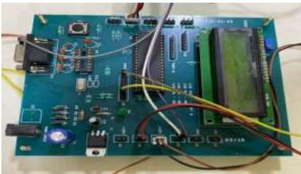
Figure 3.1.1: PIC16F877A Microcontroller
