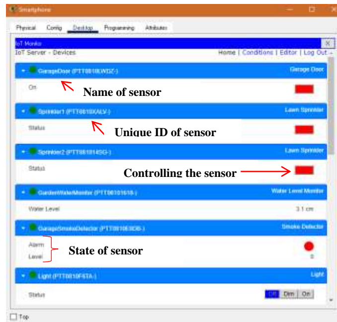
Fig 5 Monitoring and controlling smart devices
