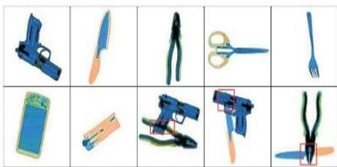
Fig 3: X-ray prohibited item images without background. The red boxes are the overlapping part of the double prohibited items. Different colors represent different materials during X-ray imaging. Blue, green and orange respectively indicate metal, mixture and organic. If the 2 items are overlapping, the color of overlapping depends with different materials are going to be covered and therefore the color of overlapping will be deepened. as an example, in figure 2, the colour of the overlap between the gun and therefore the pliers is deepened.
