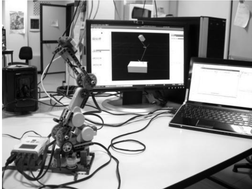
Figure 7. The LEGO robotic manipulator shown in real life and visualized through rviz .
