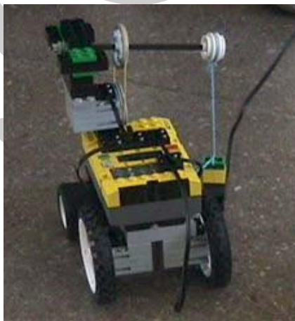
Figure 8. The RCX programmable brick with wheels, motors, and sensors (Bers et al. , 2002)
