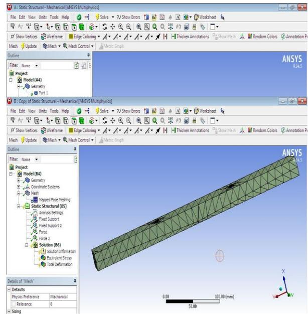
Figure 5.5 Static Structure Mesh(b).
