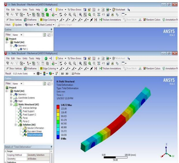
Figure 5.10 Total Deformation(a)
