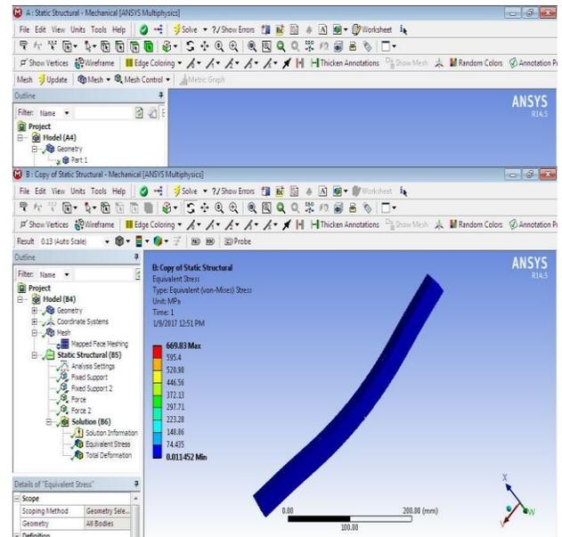
Figure 5.9 Equivalent Stress(b)
