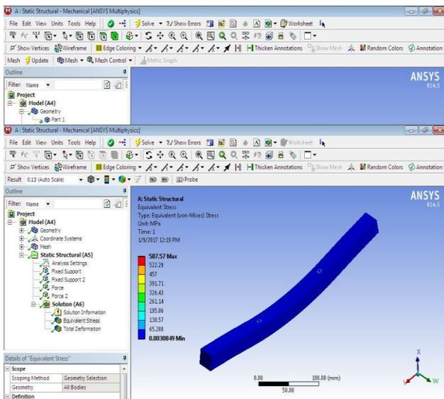
Figure 5.8 Equivalent Stress(a)
