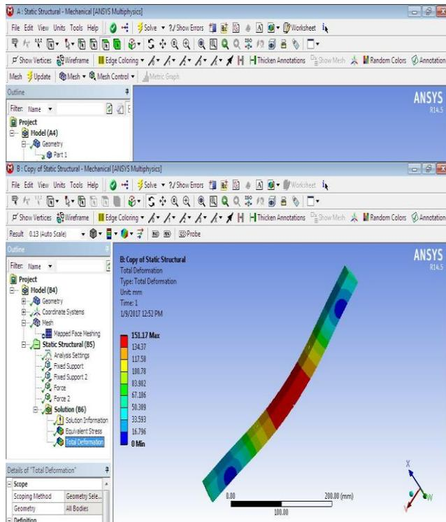
Figure 5.11 Total Deformation(b)
