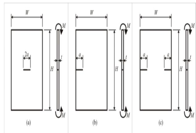
Figure 1: Geometry (a) Central cracked plate. (b) A single edge-cracked plate. (c) Double edge cracked plate.
