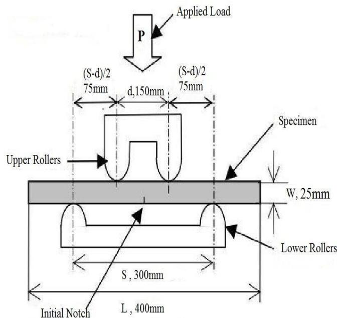
Figure 9: Experimental setup.
