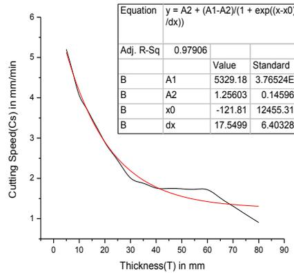
Fig.4 Effect of thickness on cutting speed
