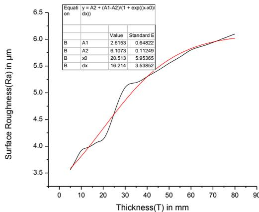
**Fig.7 Effect of job thickness on Surface Roughness**
