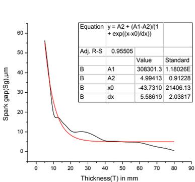
Fig. 5 Effect of thickness on Spark gap
