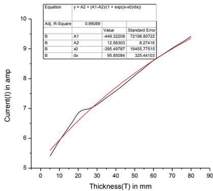
Fig.3 Effect of thickness on current
