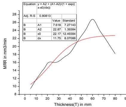
Fig.6. Effect of job thickness on MRR
