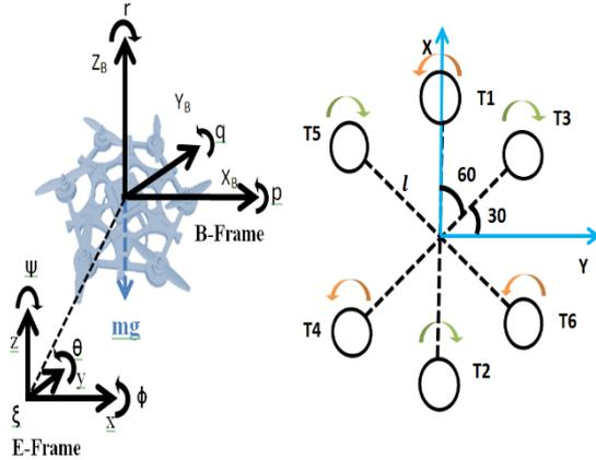
Fig 1. UAV Hexacopter structure and Frames.
