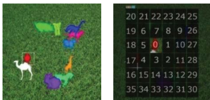
Fig. 4. A ClickAnimal image (left) and 6x6 grid (right) determined by red turkey’s bounding rectangle.
