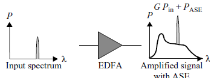
Fig. 2 Amplified Signal Spectrum with ASE
