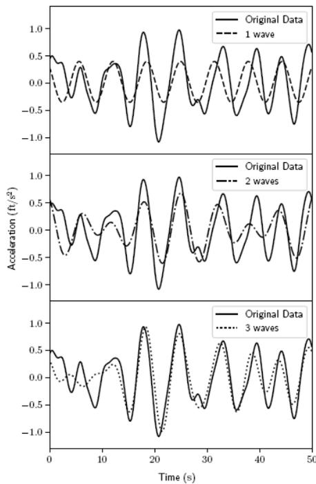
Fig. 5. The sine-summation process using three sine waves to fit a dataset.
