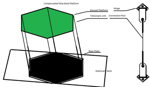
Fig. 10 – Compensated Ship Deck Platform using Stewart Platform
