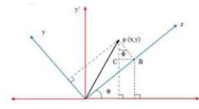
Fig.8.2 Rotation of base about y-axis
