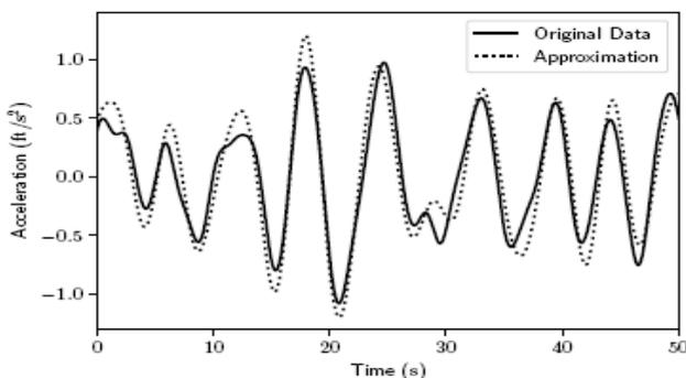
Fig. 6. The final sine-summation fit of the original data using 14 sine waves.
