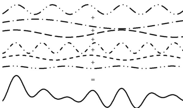
Fig. 2. Two-dimensional representation of ship deck motion.
