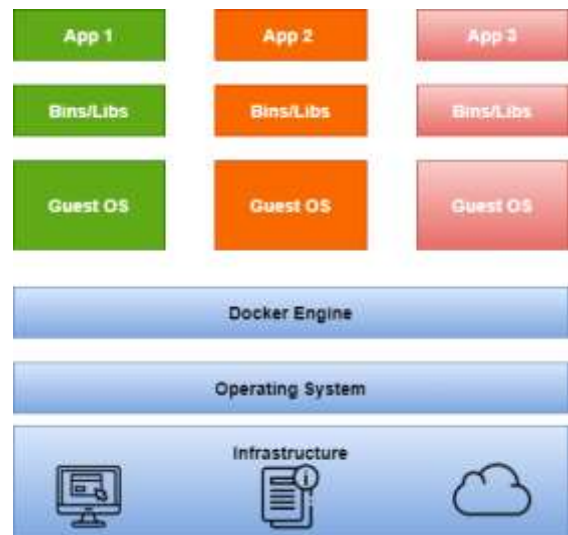
Fig. 3 Docker Container architecture
