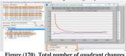
Figure (170) Total number of quadrant changes in case number Of nodes =30 and 60 / FTP application / nodes were posited gridly.
