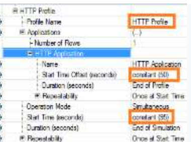
Figure (19): HTTP profile properties Used in simulation in case nodes were posited gridly, whether network was large or small
